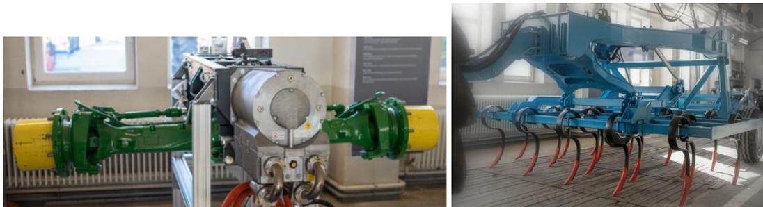
Figure 4 First prototypes of traction module (left) and tractor attached carrier with passive harrow module (right)
