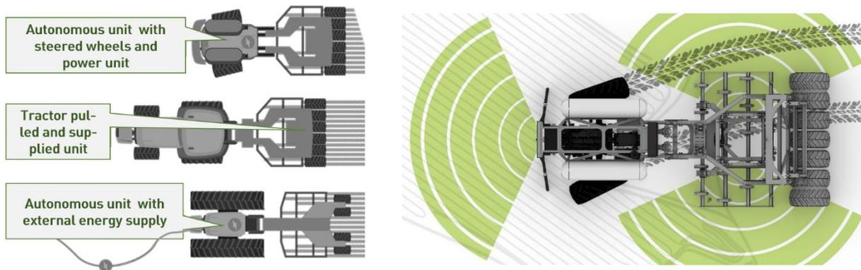
Figure 5 Basic configuration types of the Feldschwarm units
