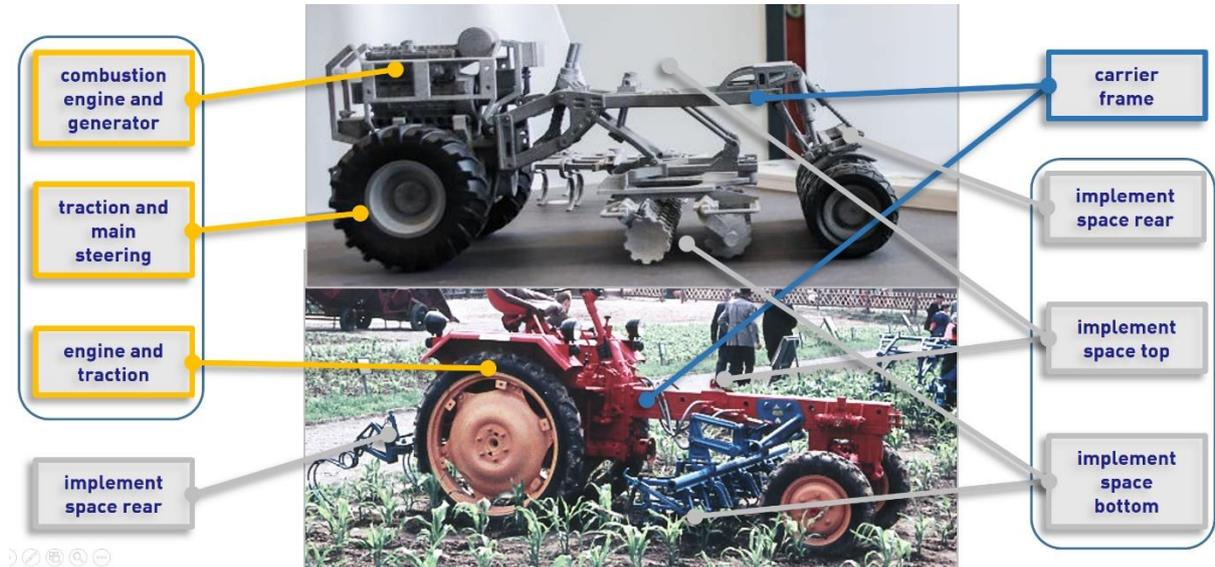
Figure 2 Modular concept of the autonomous, self-propelled Feldschwarm unit and its design similarities to a tractor from 1960 [9]
