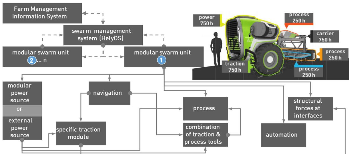
Figure 3 Tractor – implement functionality reflected in a modular system and anticipated annual usage hours for the different modules
